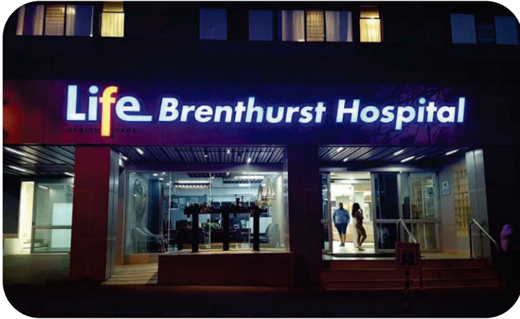
Fabricated 3D letters Aluminium return, Perspex face, Led illumination.
